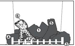
Line up the rectangular hole in the left crossover with the rectangular post located on the left side of log and install as shown. 14
