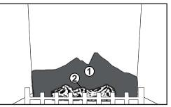
Move the charcoal strip into position lining up the holes in the bottom with the studs located on the burner on the burner. Ensure strip sits flat on the burner.
