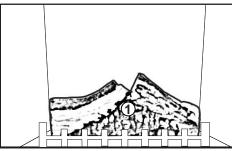
Place the rear log so that it rests against the two log brackets on the back wall of the firebox. The air space between the log and firebox back is used to facilitate combustion air flow.
