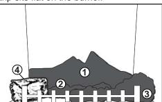
**D.** Move the left log into position lining up the hole in the bottom with the stud on the left side of the log support.
