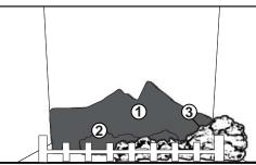
**C.** Position the front right log just behind the grate lining up the holes in the bottom with the studs located on the log support.
